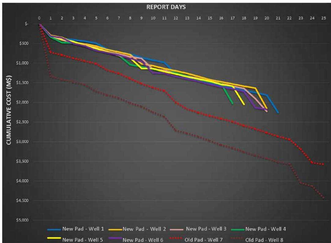
*Digital offset research resulted in a highly efficient drill plan and execution. In the above graph of Cost vs Drill Days, the new wells in the 6-well pad (solid lines) were all drilled in fewer days and at significantly less cost than Apache's two previous wells in the Ante Creek area (dotted lines).*
